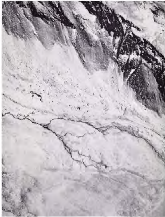
FIG. 10. Sample black-and-white photograph, 1:10,000, f=6 inches. Compare with the photograph on the Front Cover which is of the same area taken on Kodak Ektachrome Aero Film, Type 8442, from a Cibachrome print (direct positive process). (Courtesy CIBA Photochemical Ltd., Basel, Switzerland.)
