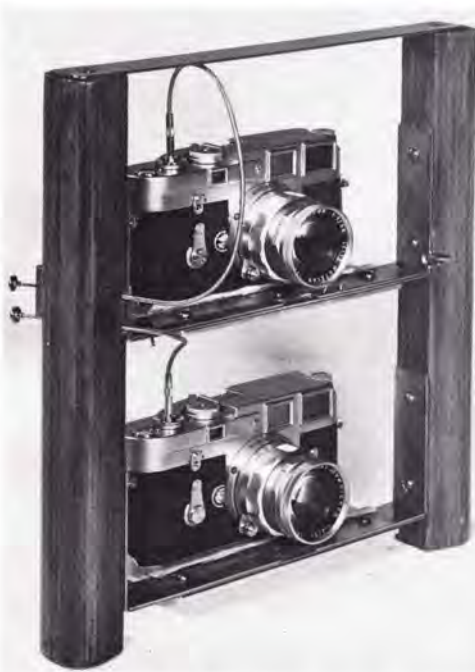
FIG. 10. Paired camera arrangement for making simultaneous photographs.
