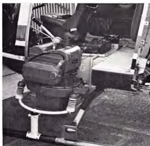
FIG. 1. The aerial camera is mounted outside the cabin using special vibration-damping fixtures.
