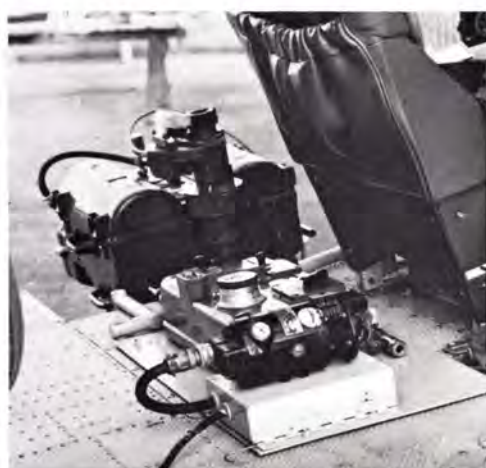
FIG. 2. The camera control box and vacuum pump are located on the floor inside the cabin.
