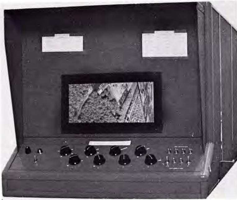
FIG. 4. Multispectral additive color viewer.
