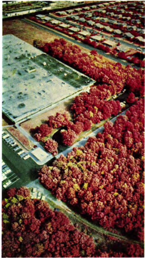
PLATE 2b. A composite false color rendition of green, red, and infrared spectral photographs (enlarged 35 mm. color negative reproduction of viewer screen).
