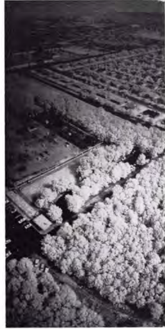
PLATE 1d. Spectral photograph in the near infrared band (700 to 980 nm.).
