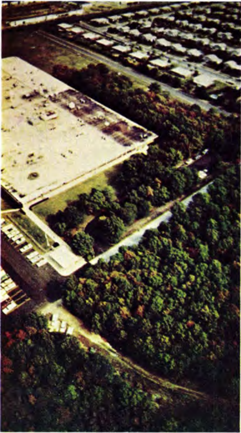
PLATE 2a. Composite "true" color rendition of blue, green, and red spectral photographs (enlarged 35 mm. color negative reproduction of viewer screen).
