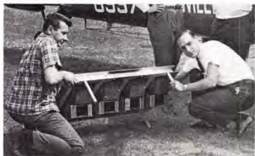
FIG. 2. A four-camera rack of optically aligned KA-56 cameras showing external mountings of the filters.
