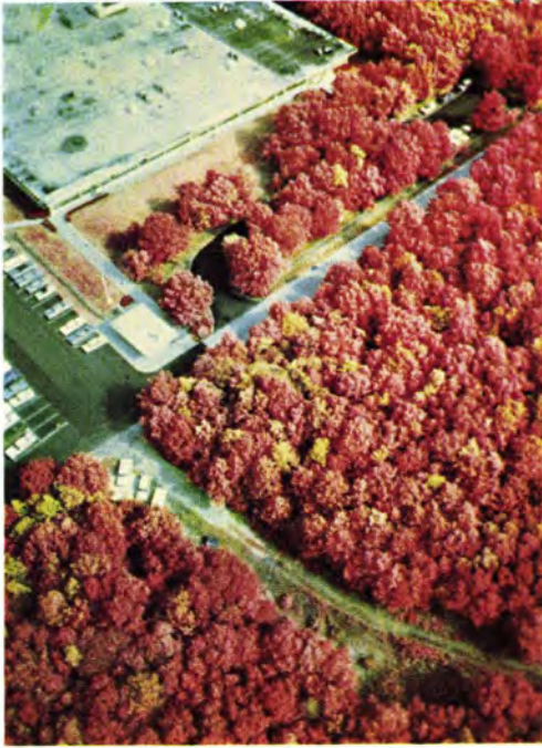
PLATE 3a. Standard camouflage detection false color rendition using green, red, and infrared spectral photographs.
