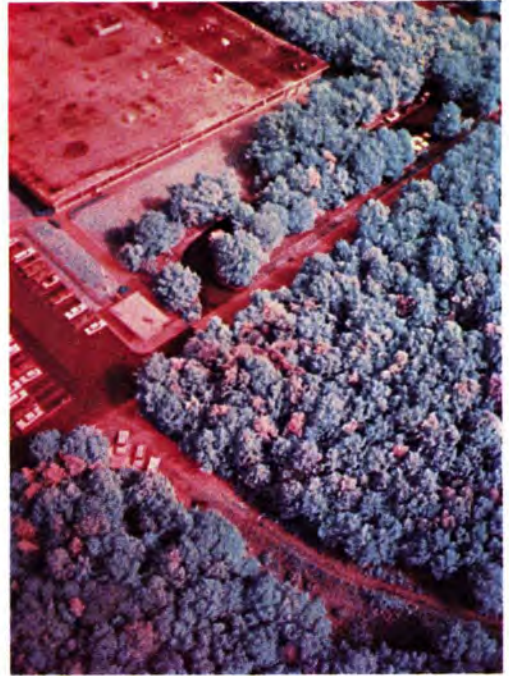
PLATE 3b. False color space using four spectral bands which exhibit improved color separation.
