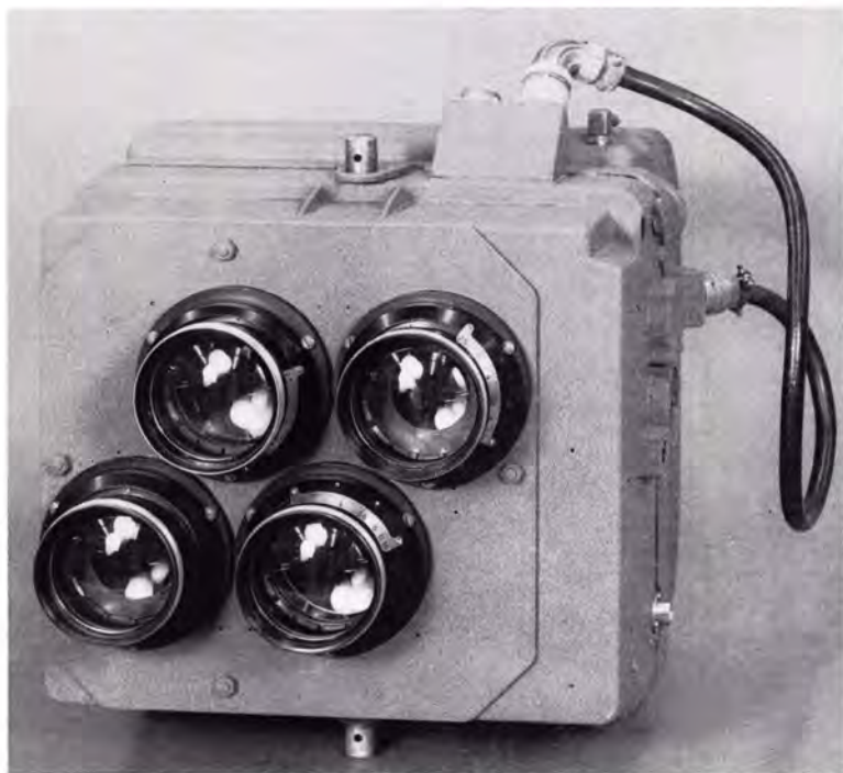
FRONTISPIECE. Four-lens multispectral camera used for research. See page 1026.
