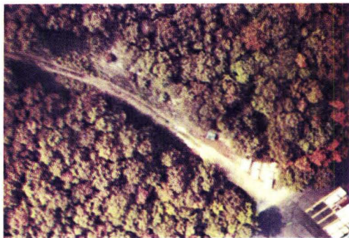
PLATE 4b. False color target detection mode showing chromatic enhancement of vehicle and suppression of natural background.
