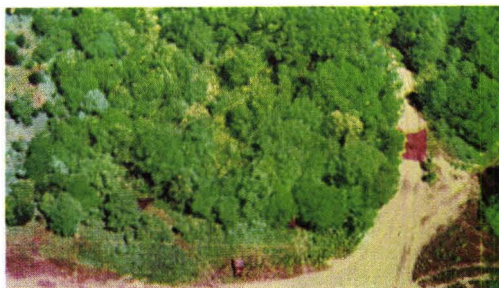
PLATE 4d. Multispectral color presentation of test site. Note detectability of camouflage nets in trees.
