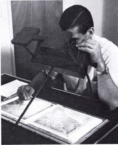
FIG. 3. A photo interpreter uses an Old Delft stereoscope and desk-type fluorescent light table to study an aerial photograph.
