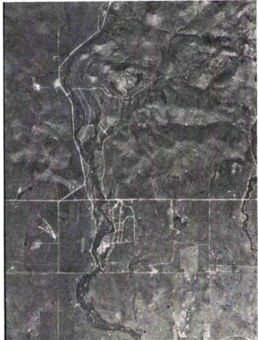
FIG. 5. Orthophoto: camera altitude, 25,000 feet; focal length, 6 inches; scale of output, 1:50,000.
