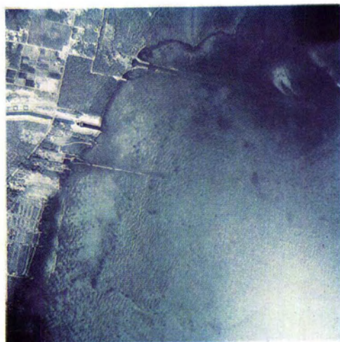
PLATE IV. Shoreline area east of Cutler, Florida showing areas of fresh-water discharge; from regular color transparency at original scale of 1:12,000.
