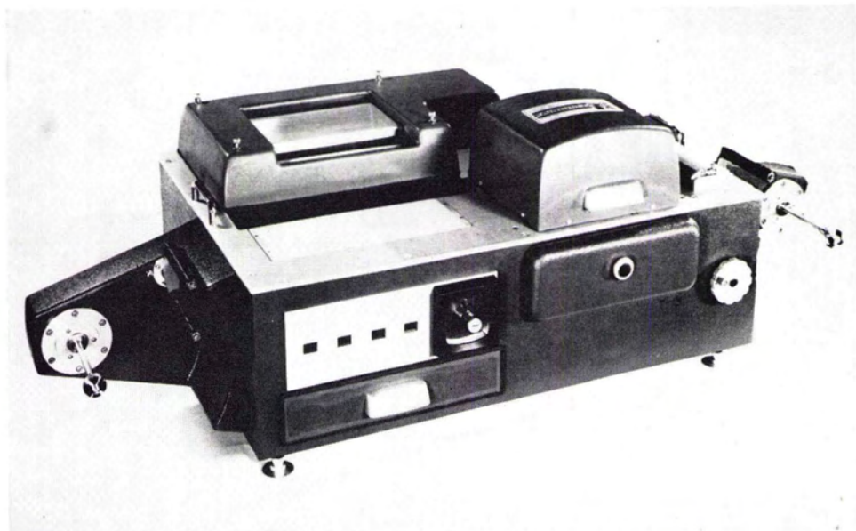
FIG. 1. Fairchild field rectifier for 3-inch focal-length panoramic photography.
