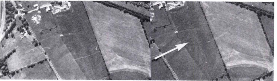
FIG. 15. A field of corn classified as FAIR exhibits an irregular or coarse textural stereo pattern on the field (arrow). Relief in the height of the corn is more constant than that of the poor fields, but zones of slightly stunted stalks can still be detected. In many cases a good number of missed-rows leave gaps in the row pattern. In this classification no zones of bare soil are visible because of complete vegetation cover. However, areas of less vigor do exist and are identified by their lower relief. This field measures 20.5 acres and produced 246 tons of silage corn, or 10.8 tons per acre.
