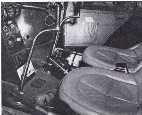
FIG. 3. Cockpit of the helicopter showing the installation of the vacuum pump in the center background.
