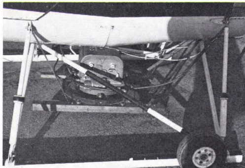
FIG. 2. The helicopter mount is relatively simple, consisting of angle iron members, and straps suspended from strut.
