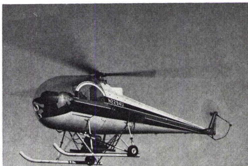
FIG. 1. Fairchild Cartographic camera mounted underneath a helicopter.
