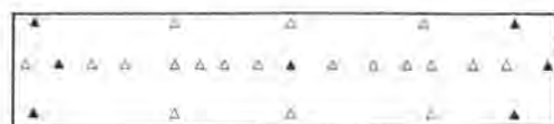
FIG. 4. The nine-model strip. Triangles denote ground control points, and black triangles denote those control points that were used in the adjustment.
