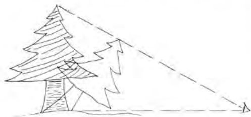
FIG. 1. Error in height measurement introduced by tree lean or sway.
