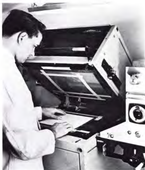
FIG. 1. The LogEtronics Mark III Color Contact Printer contains a printing light consisting of a modulated scanning beam on a special tri-color phosphor cathode-ray tube.
