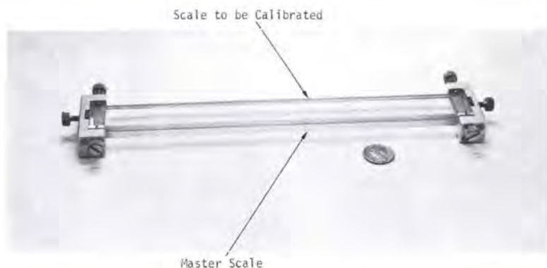
FIG. 5. Alignment device used in calibration of scales against master scale.
