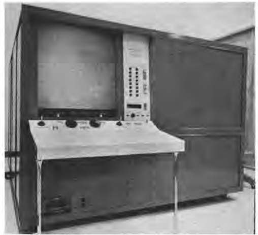
FIG. 10. Mensuration equipment used on Project RAMP included this Gilleland Point Coordinate Mensurator, a partly automated type of comparator.
