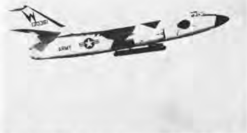
Fig. 2. The YEA-3A twin engine jet aircraft with the radar antenna contained in the pod beneath the fuselage.
