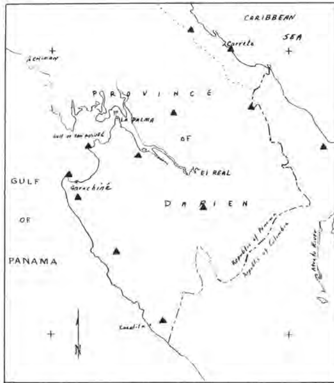
FIG. 3. Sketch of Darien Province showing the locations of the radar reflectors that served as control points.
