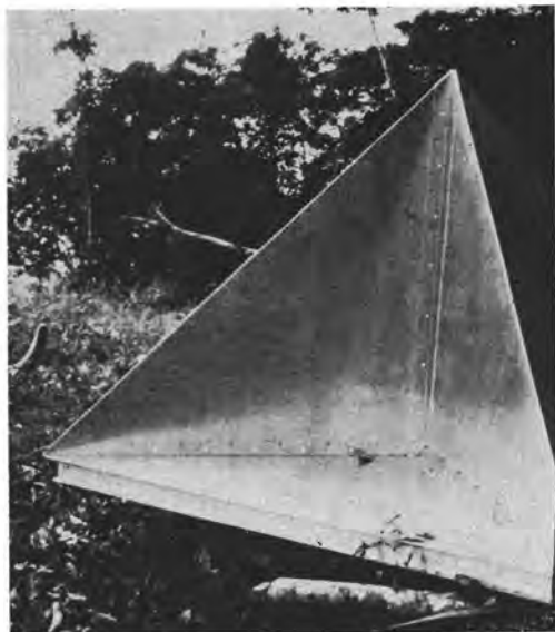
FIG. 4. A radar reflector consisted of a cluster of four corner reflectors measuring 5.5 feet on a side and 3.9 feet high and weighing 150 pounds; the unit was disassembled for convenience in carrying.
