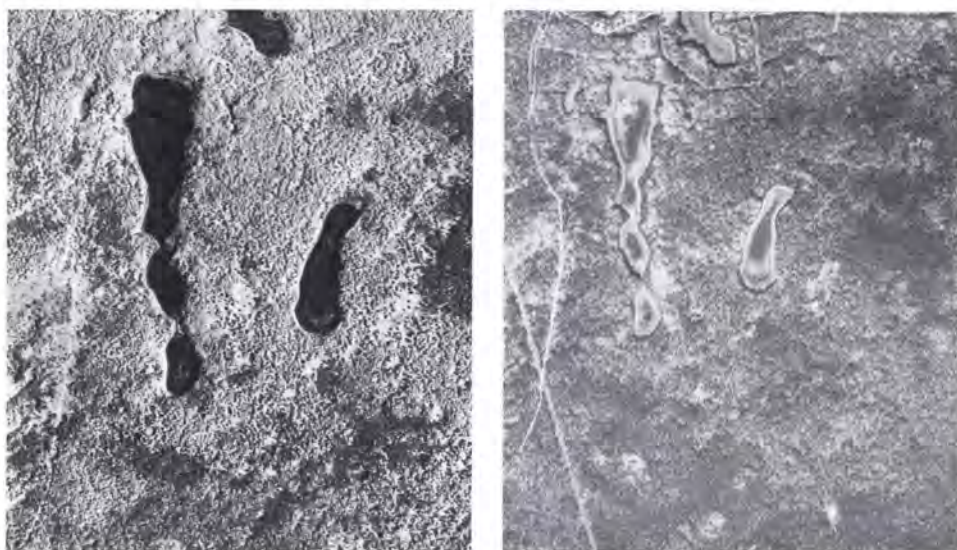
FIG. 3. Modified infrared (left) and panchromatic air-photos of a shallow lake in Otsego County, Michigan. A regional drop in the water table between 1952 (left) and 1964 caused the lake nearly to dry up (USDA photo).
