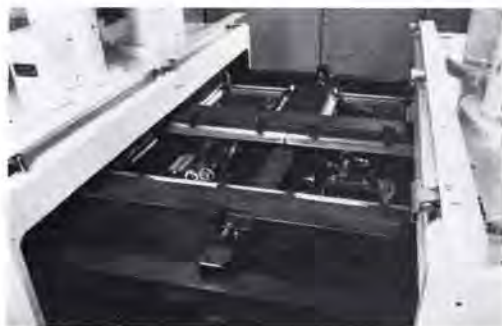
FIG. 6. Automatic Photomapper table (showing master carriage, two positionable diapositive lenses, and two fixed output lenses).
