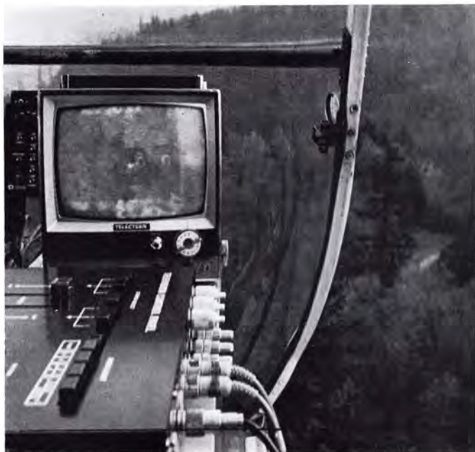
FIG. 2. Slung beneath the helicopter, an Ampex closed circuit TV camera captures video images for the monitor mounted in the cockpit. The camera provides a view of the trees being examined while the results of that examination—the temperatures of the trees taken by a heat-sensing device—are indicated by the numbers registered on the monitor screen by a second camera. (Photo by Gregg Perry.)
