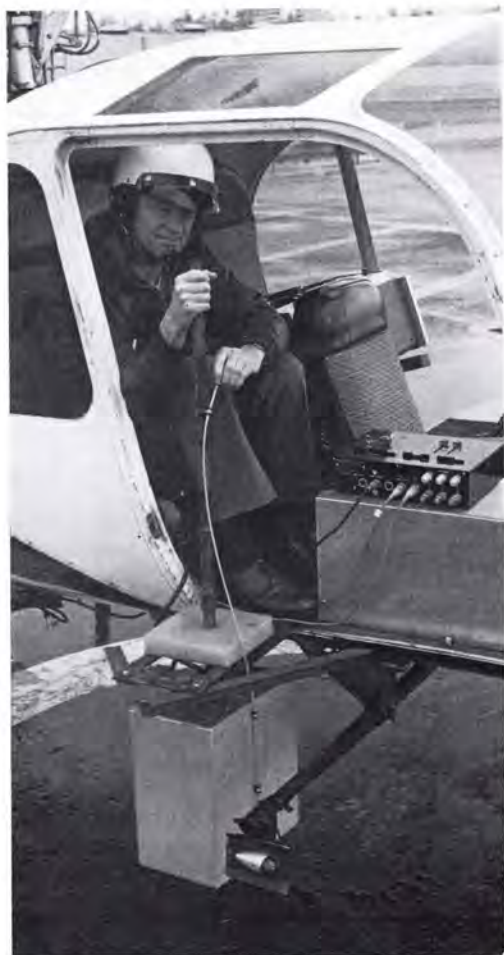
FIG. 1. John Wear of the USDA Forest Service's Pacific Southwest Forest and Range Experiment Station prepares the equipment that is to be used to take the temperature of trees. The pod attached to the lower frame of the helicopter contains a heat-sensing unit and a closed circuit TV camera. (Photo by Gregg Perry.)
