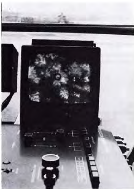
FIG. 3. A close-up view of the television monitor shows (circled) the tree being measured for heat generation, and the reading (the number 4) indicated on the counter. A picture of the trees and the temperature information are recorded on an Ampex videotape recorder for later study. (Photo by Gregg Perry.)
