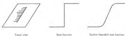
FIG. 3. Target Edge, Step Function, and System Degraded Step Function.
