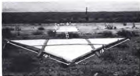
FIG. 2. Part of a target array, showing a triangular central target and one of the wing panels.
