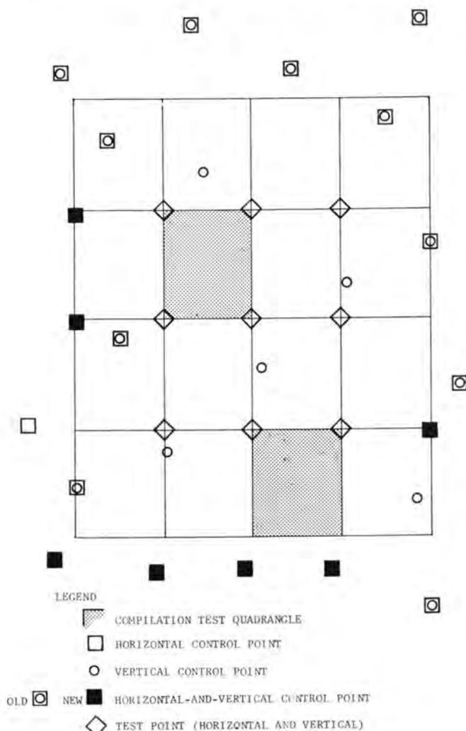
FIG. 1. Control and test points for the Tucumcari Project
