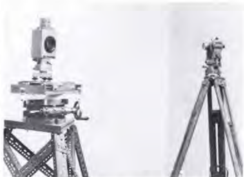
FIG. 2. The camera and the theodolite for the observation and intersection of the projections of the outer perspective center.
