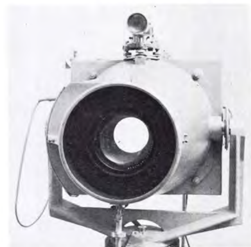
FIG. 4. The image of the diaphragm for the f -stop 1:6.3.
