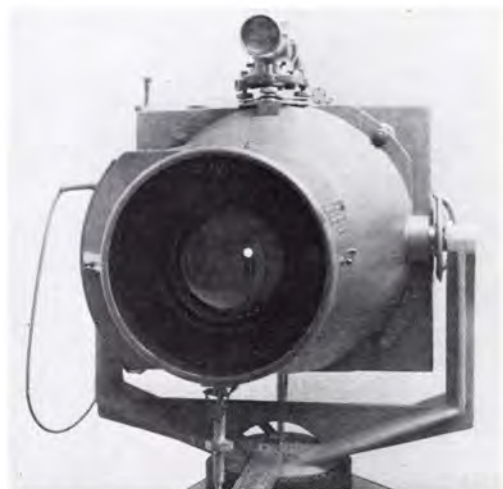
FIG. 3. The outer perspective center to be observed and projected on the outside of the camera with three or more theodolites. f -stop 1:70.
