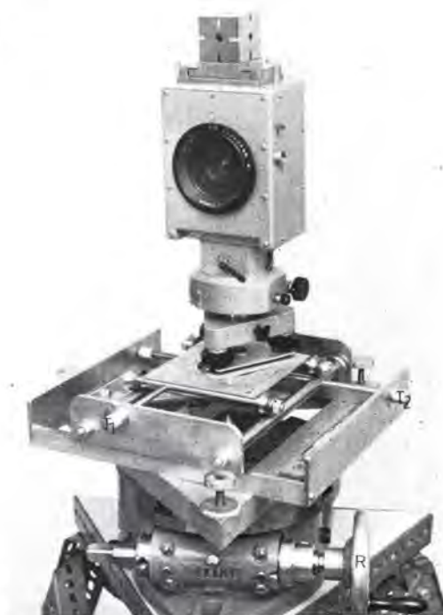
FIG. 1. Terrestrial survey camera (Zeiss TMK) placed on a table for the location of the perspective centers. The camera can be translated with the screws T1 and T2 and rotated with the screw R . The table can be levelled with three foot-screws
