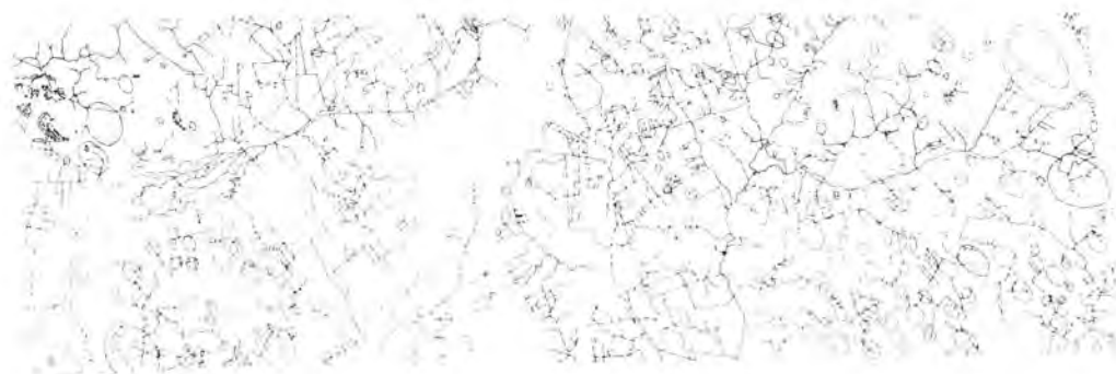
FIG. 2. Drainage map prepared from Ektachrome infrared photographs, Bennettsville, S. C., Test Area.
