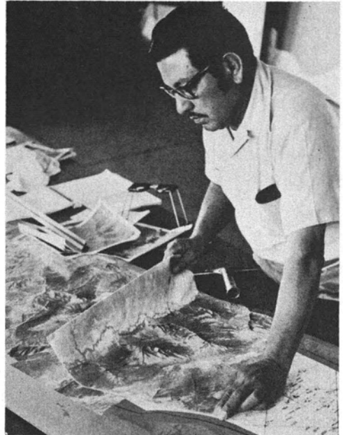
FIG. 3. Mosaicking area photographs to form a larger picture of the ground covered, this employee uses a contour map as a base on which he mosaics. The aerial pictures overlap 60 percent so that each picture in a series contains parts of another. In preparing a mosaic, the employee uses only the central parts of each photograph.
