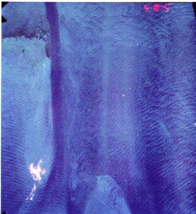
Simulation of Ektachrome Infrared type 8443 using multispectral records 4, 6, and 7 printed blue, green and red, respectively.
