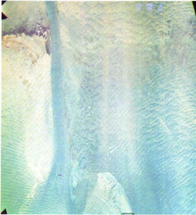
Simulation of normal camera original color tripack using multispectral records 1, 4, and 6 printed blue, green, and red, respectively.
