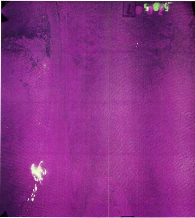
Bicolor presentation of record 1 (400-460 nm) printed blue and red with record 7 (685-900 nm) printed green. Sea state and surface detail recorded with very little depth information.
