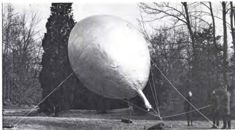
FIG. 13. A hydrogen-filled balloon of 700 cubic feet moored in a wind of 20 miles per hour prior to a test flight in Connecticut.
