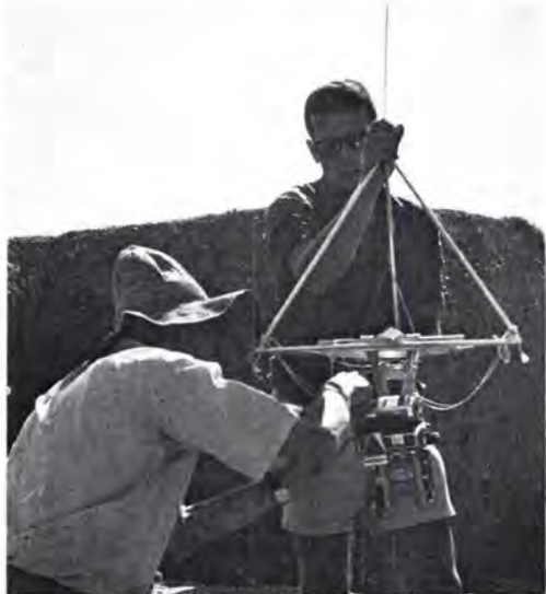
FIG. 2. Hanging the camera preparatory to a balloon flight.
