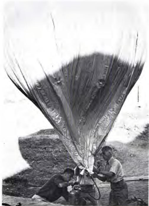
FIG. 1. Filling a tethered balloon to carry an aerial camera.
