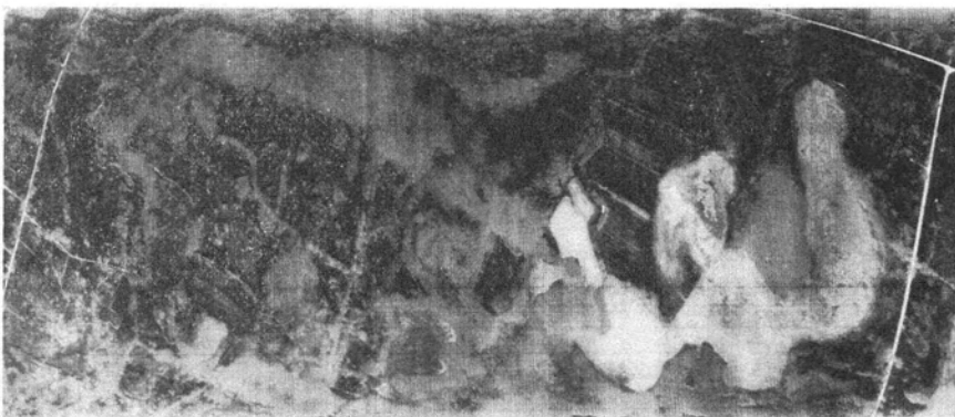
FIG. 3. Infrared imagery in the 0.7 to 14 micrometer wavelength band obtained at night from 1000 feet on 17 July, 1968. None of the girdled trees were detectable without prior knowledge of their locations.
