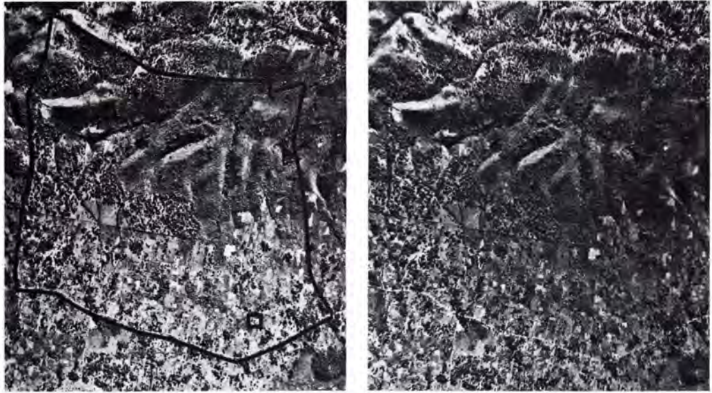
FIG. 2. Estimates of unenumerated population totalling several hundred and various demographic characteristics in the district shown were made by air photo interpretation. Care was needed to distinguish in this semi-arid area small homes from large water cisterns and catchments (small square shows one of each).
