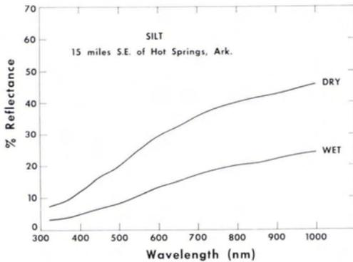
FIG. 3. Type 2 curves for a sample of pedalfer-type silt.
