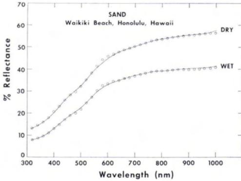
FIG. 24. Type 2 curves for a carbonate sand sample.
