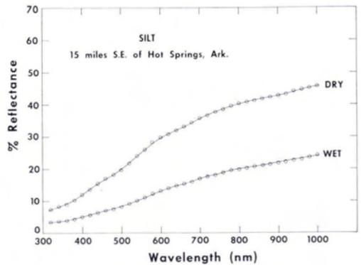
FIG. 9. Type 2 curves for a sample of pedalfert-type silt. Measured values are shown by lines; predicted values by a series of circles.
