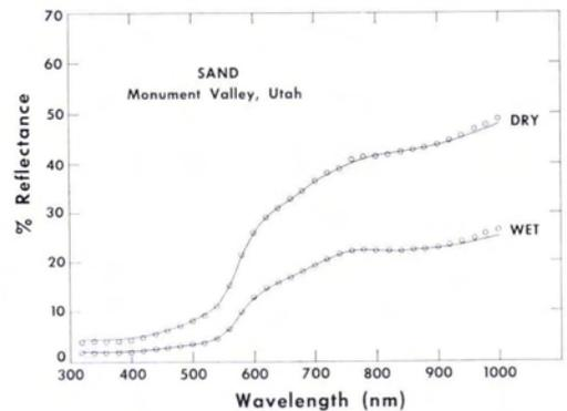
FIG. 10. Type 3 curves for a sample of red quartz and calcite sand. Measured values are shown by lines; predicted values by a series of circles.
