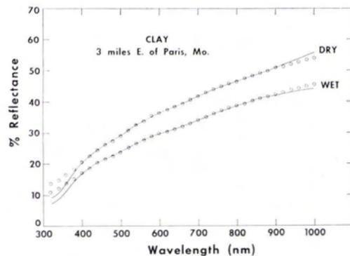
FIG. 22. Type 2 curves for a clay sample. Note that the difference in reflectance between the dry and wet curves in this figure is fairly small.
