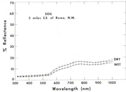
FIG. 30. Type 3 curves for a sample of a very low reflectance, pedalfert-type soil. Note the very small difference in reflectance in the wet and dry curves.
