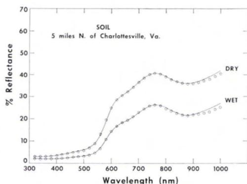
FIG. 11. Type 3 curves for a sample of laterite-type soil. Measured values are shown by lines; predicted values by a series of circles.
