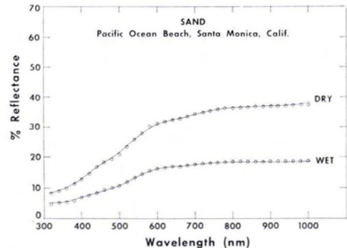
FIG. 17. Type 2 curves for a sample of quartz and rock-fragment sand.
