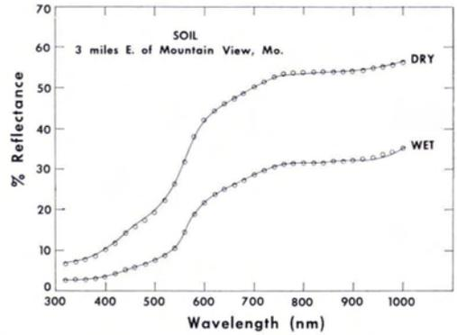
FIG. 25. Type 2 curves for a pedalfert-type soil sample.
