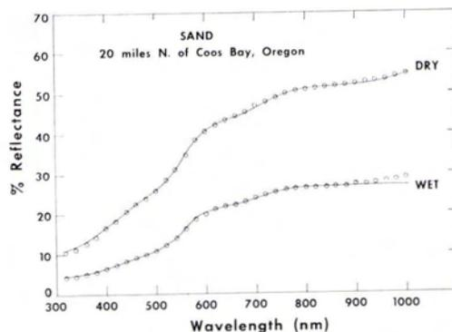
FIG. 23. Type 2 curves for a sample of quartz sand.
