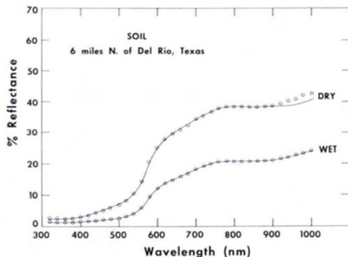
FIG. 35. Type 3 curves for a sample of a pedalfert-type soil.
