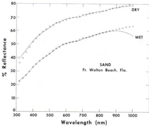
FIG. 29. Type 2 curves for a sample of quartz sand, collected at Ft. Walton Beach, Florida. This sample was found to have the highest spectral reflectance of any thus far measured, reaching a value of 79 percent at 1,000 nm.
