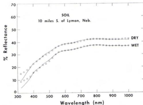
FIG. 21. Type 2 curves for a pedocal-type soil sample. Note the small difference in reflectance between the dry and wet curves.
