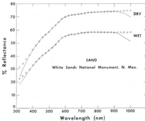
FIG. 28. Type 2 curves for a sample of gypsum sand. Note that beyond 920 nm there is a sharp decrease in the reflectance for both the wet and dry curves, the abridged technique was unable to predict correctly values beyond 920 nm.
