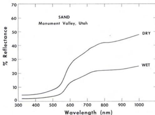
FIG. 4. Type 3 curves for a sample of red quartz and calcite sand.
