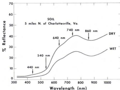
FIG. 7. Location of the five selected wavelengths with respect to the curve shape of one of the soil samples.
