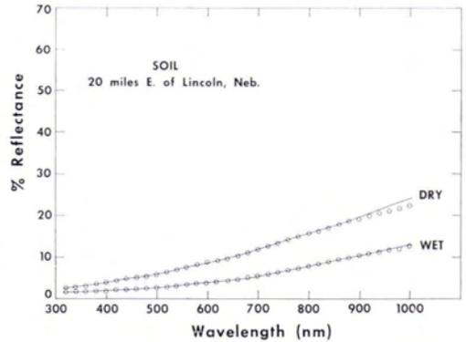
FIG. 8. Type 1 curves for a sample of chernozem-type soil. Measured values are shown by lines; predicted values by a series of circles.
