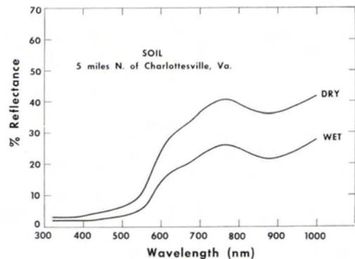
FIG. 5. Type 3 curves for a sample of laterite-type soil.
