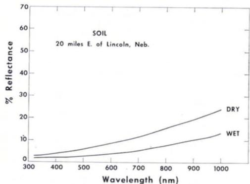
FIG. 2. Type 1 curves for a sample of chernozem-type soil.
