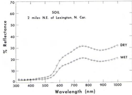
FIG. 32. Type 3 curves for a sample of a laterite-type soil.
