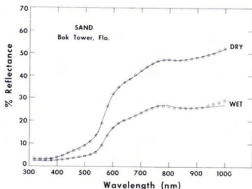
FIG. 37. Type 3 curves for a sample of quartz sand with a hematite stain.
