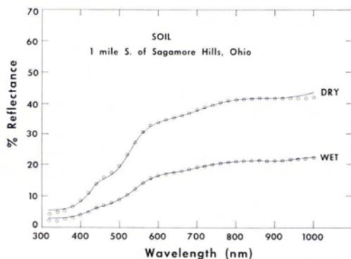
FIG. 20. Type 2 curves for a pedocal-type soil sample.
