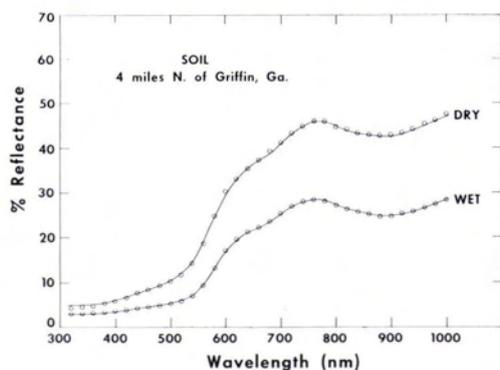
FIG. 36. Type 3 curves for a sample of a pedalfert-type soil.
