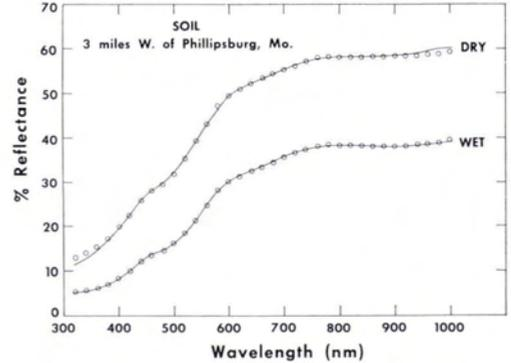
FIG. 27. Type 2 curves for a pedocal-type soil sample of very high reflectance.
