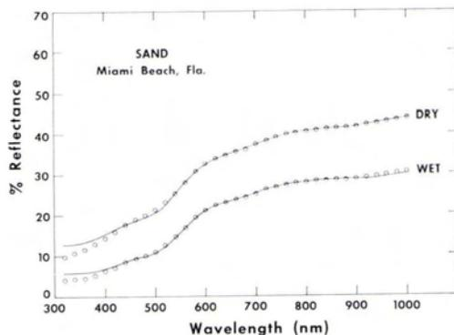
FIG. 19. Type 2 curves for a sample of quartz and carbonate sand.
