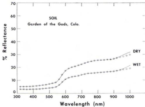
FIG. 31. Type 3 curves for a sample of a pedalfert-type soil.
