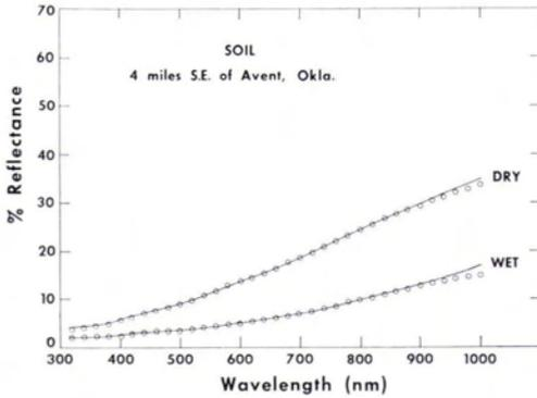
FIG. 14. Type 1 curves for a sample of chernozem-type soil
