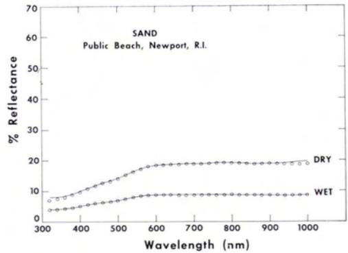
FIG. 15. Type 2 curves for a sand sample containing quartz, rock fragments, and shell fragments. The unusual feature of these curves is that they are flat over such a long wavelength span: 600 to 1,000 nm.
