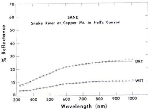
FIG. 16. Type 2 curves for a sample of quartz and rock-fragment sand.
