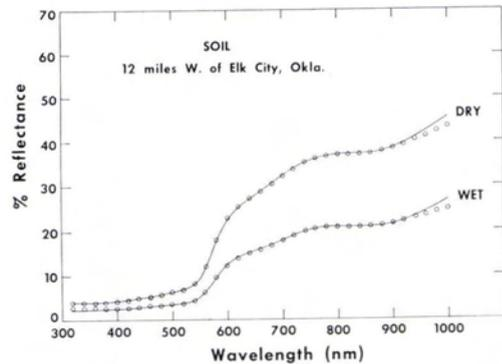
FIG. 34. Type 3 curves for a sample of a pedocal-type soil sample.
