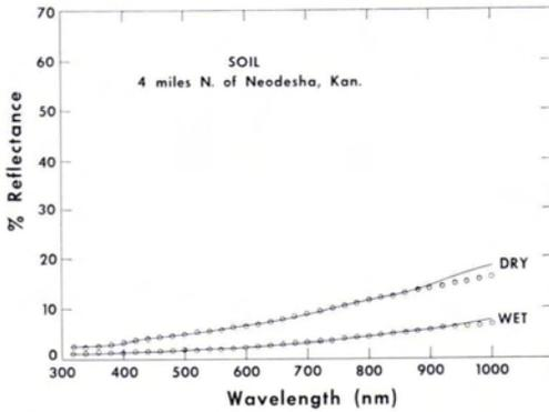
FIG. 12. Type 1 curves for a sample of chernozem-type soil. Measured values are shown by lines; predicted values by a series of circles.
