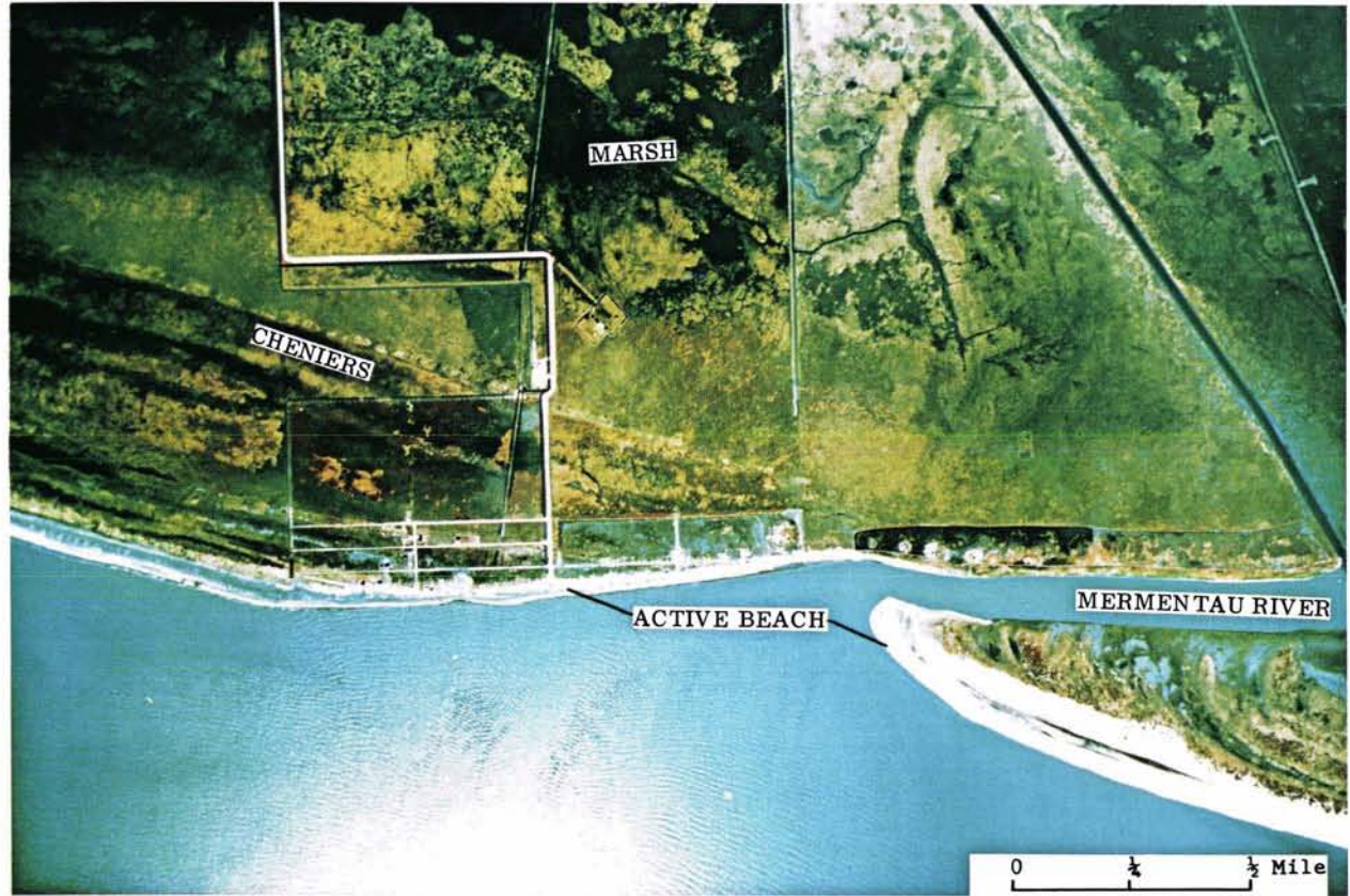
PLATE 1. Color infrared photograph of the active beach in Area 19 at the mouth of the Mermentau River. The beach (white in tone) is composed of a mixture of sand and shells. The arcuate ridges on the seaward side of the river indicate successive deposition of sediments which are extending the river mouth to the west. Near-shore wave patterns indicate the presence of sub-surface bars.
