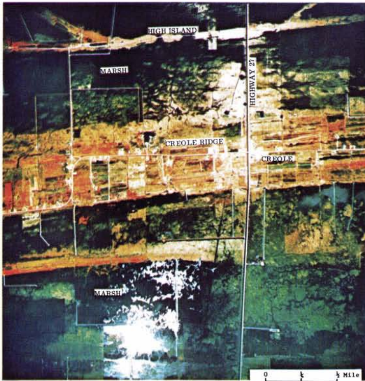
PLATE 2. Color infrared photograph of Creole Ridge and High Island in Area 19. The reddish tones produced by the grasses growing on the ridges contrast sharply with the dormant marsh vegetation. These ridges are predominantly composed of shells but locally contain sand lenses.
