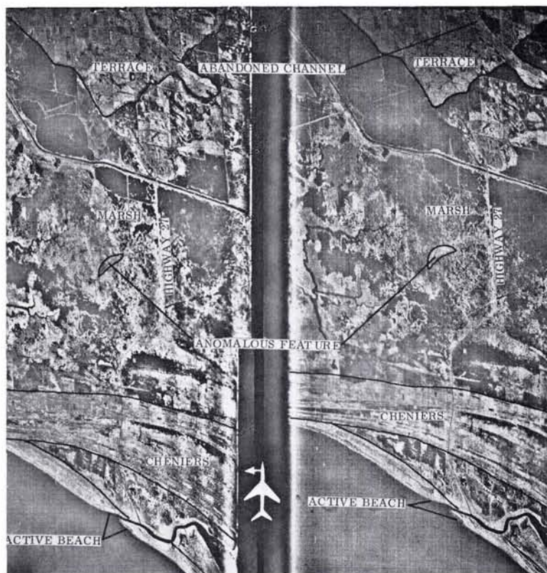
FIG. 5. APQ-97 radar imagery of the western half of Area 19. Compare the major physiographic units with those delineated on the photo index (Figure 3). Note the return from the crescent-shaped anomalous feature on the HV channel (right) as compared with the HH channel (left). The original scale was approximately 1:200,000.
