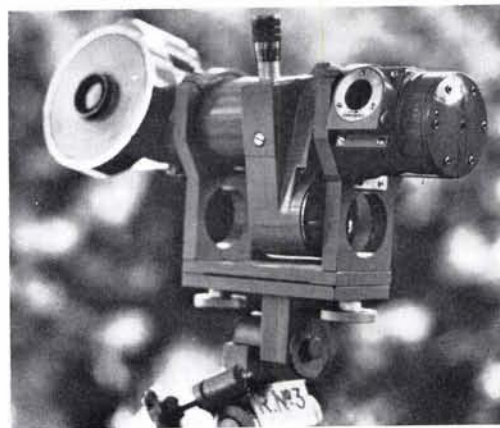
FIG. 12.—Ground crew used a Barr and Stroud optical dendrometer to measure the boles of 4 to 6 trees on each selected ground plot.
