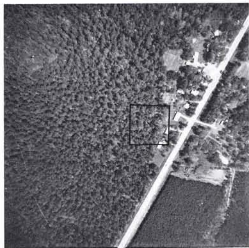
FIG. 10. This 1:12,000-scale photograph covers the area outlined in white in Figure 9. The area outlined in black corresponds to the coverage of the 1:2,000 scale photography shown in Figure 11. Each sample strip was completely covered by 1:12,000 photographs. The photo shown is a 2.2× enlargement made from negative color film.
