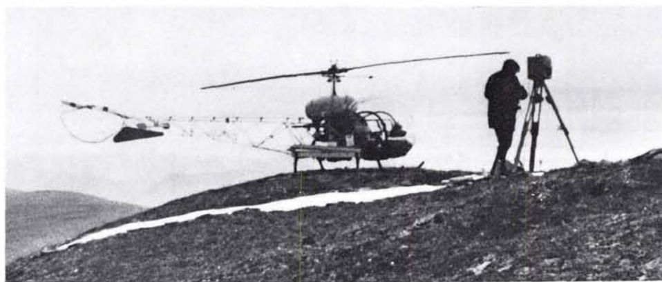
FIG. 1. George Brennan, Geotronics' Chief Surveyor on the TAPS Project, operates MRA-3 Tellurometer on Alaskan mountain top. Note leg of control panel across center of picture.
