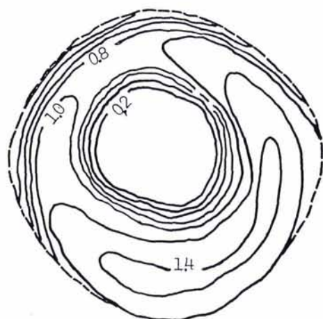
FIG. 4. Contour map of the stereo pair of Figure 3 plotted with a Zeiss Stereotope (blood cell only). Compilation scale 10,000:1. The contour values are in micrometers.
