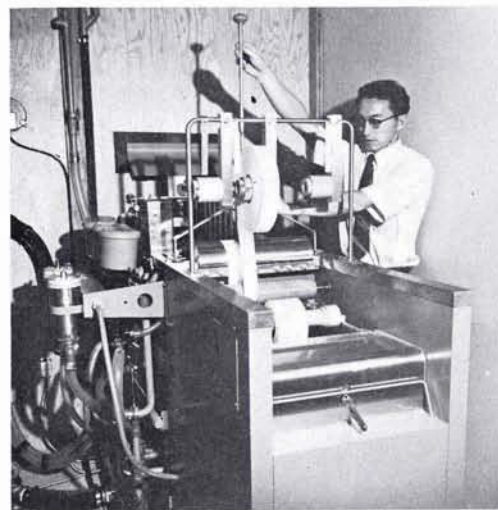
FIG. 3. The rolls of Kodak Professional color paper are processed in the Department's Model 4C3 continuous print processor.
