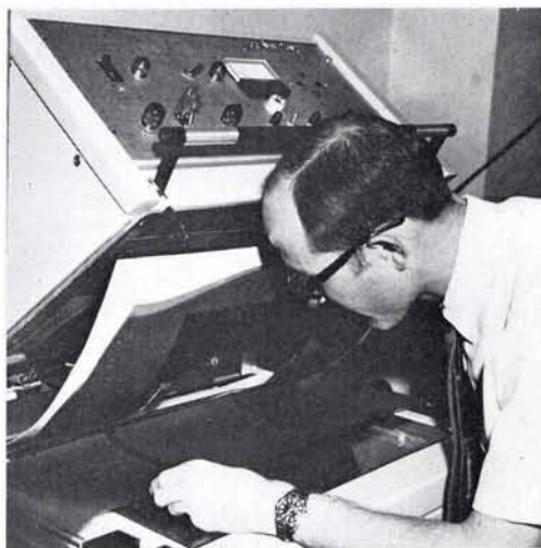
FIG. 1. A LogEtronics Mark II Electronic Contact Printer is used for volume production of black-and-white prints in the Photography and Reproduction Departments of the Surveys and Maps Branch. Average annual production of 9×9-inch black-and-white contact prints has been between 50,000 and 60,000.
