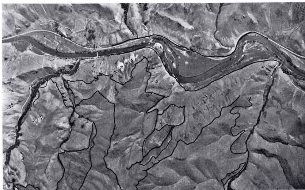
PLATE 3. Another black-and-white print made from the same color negative as Plate 5 on which a U.S. Forest Service soil scientist has mapped the soil in the overlapping portion of stereopairs using a mirror stereoscope.
