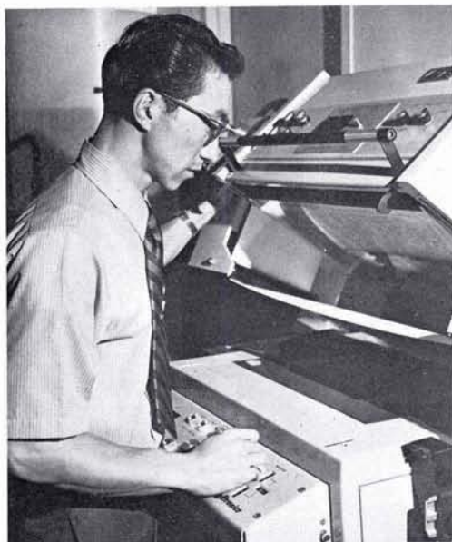
FIG. 2. A LogEtronics Mark III Color Contact Printer is being set up to expose a frame from an aerial roll negative. The 9½-inch wide roll of paper is mounted on an automatic roll transport capable of accepting 1,000-ft rolls. The printing paper is advanced the required print width automatically when the platen of the printer is lifted after exposure, as the operator is doing here. Nominal output of the Mark III printer is from 250 to 300 production prints per 8-hour day, including time for test prints.
