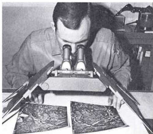
FIG. 4. A U.S. Forest Service ranger is using a mirror stereoscope to study a color stereopair of a forest area he manages.
