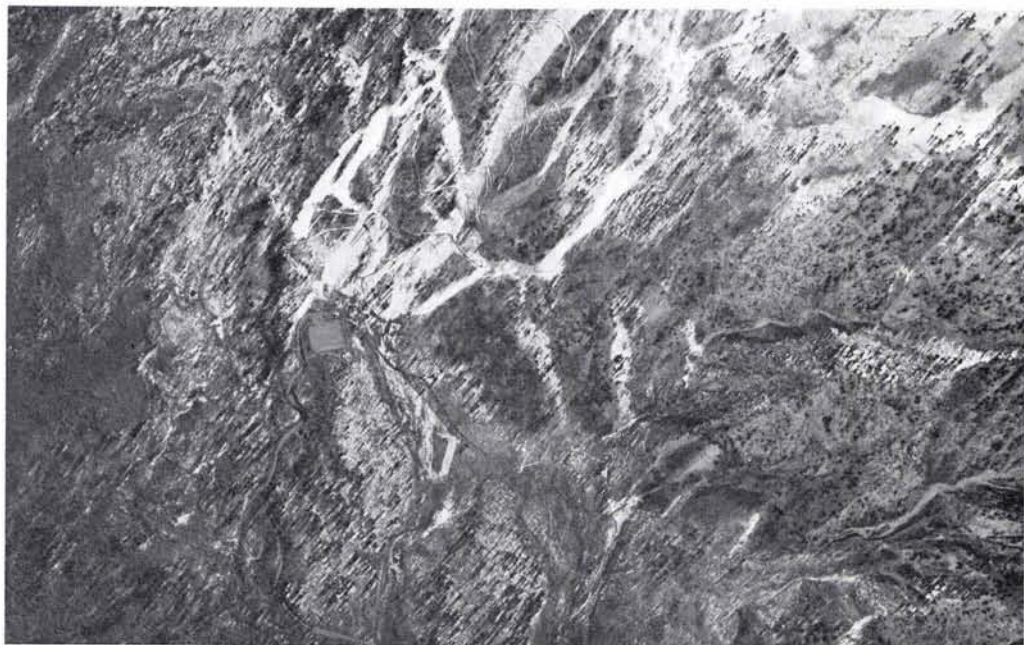
PLATE 1. Portion of aerial photograph showing Snow Basin in Utah. The original scale was 1:15,840 and this is approximately 1:20,000. The original photograph was an aerial negative, Ektachrome MS 2448 film (Plate 4). This print was produced with a multiple-lamp black-and-white printer.
