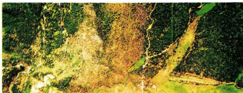
Figure 14. Serpentine area of Bucks Lake, California 28,000 feet above sea-level. The green band projected as blue, red band projected as red, the infrared band projected green.
