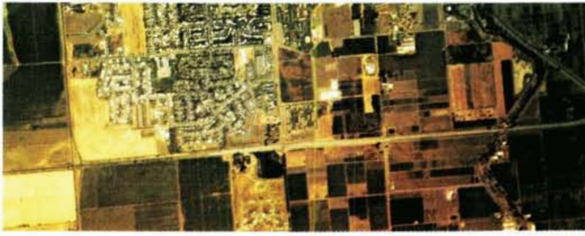
Figure 7. A multispectral true color rendition copied from the viewer screen in which the blue, green and red multispectral positives are projected each in the same color.
