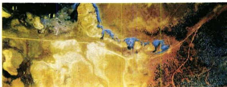
Figure 16. Harvey Valley, California 28,000 feet above sea-level false color rendition. Green band projected as green, red band projected as red, and the infrared band projected as blue.
