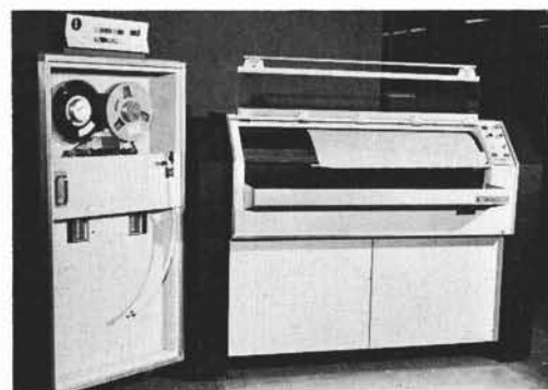
FIG. 2. IBM drum scanner (right) showing the 4-by-4-foot sheet preparatory to scanning, and the tape drive on the left.
