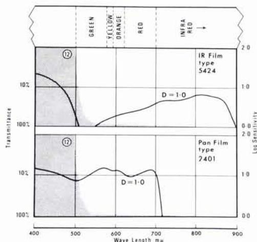
FIG. 1. Spectral sensitivity curves for Kodak film types 5424 and 2401 and Wratten No.12 filter.
