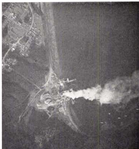
FIG. 1. Aerial photograph taken with a Hasselblad camera from 10,000 feet during a 4-knot wind in color (shown here in black and white).
