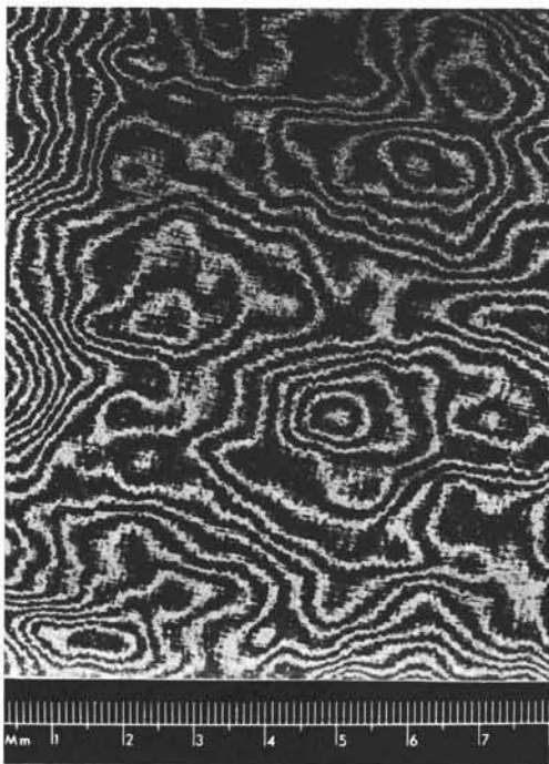
FIG. 7. Thickness fringes from triacetate film base, showing minute linear features on the emulsion surface.
