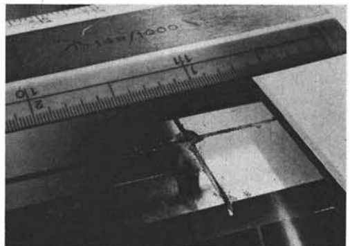
FIG. 12. Vacuum slot for film-edge retention.
