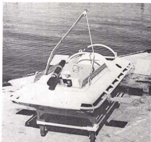
FIG. 1. RUFAS (Remote Underwater Fishery Assessment System) is a vane-controlled vehicle, flies with video and photographic cameras to record scallops during resource surveys.
