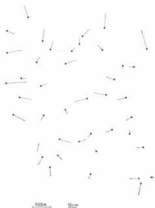
FIG. 9. External block adjustment. Residuals given at n=42 horizontal control points.
