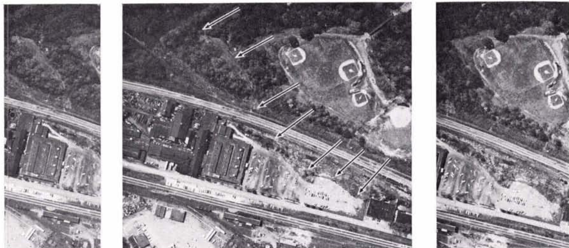
FIG. 7. Outfall detectable from drainage pattern. Arrows follow drainage pattern from river bank, under railway tracks, to approximate source.
