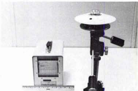
FIG. 2. Eppley Model 2 pyranometer and ICA Model 400 recorder used to measure global solar radiation.
