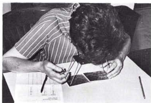
FIG. 3. Photo interpretations were made from 3 x 5-inch Kodacolor-X color prints with a standard pocket stereoscope.
