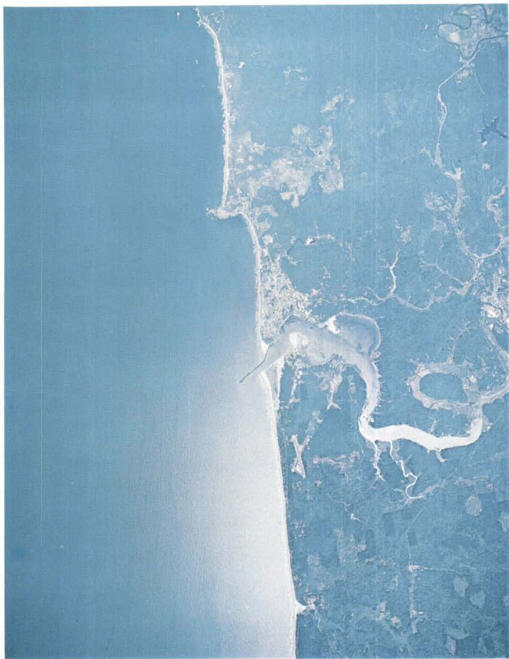
PLATE 10. High-altitude Ektachrome showing effluent trail from a pulp mill outfall located north of the Newport jetty. Discolored water appears to be entering Yaquina Bay on the flooding tide. Note also the turbid water seen along the coast in the top of the photograph.
