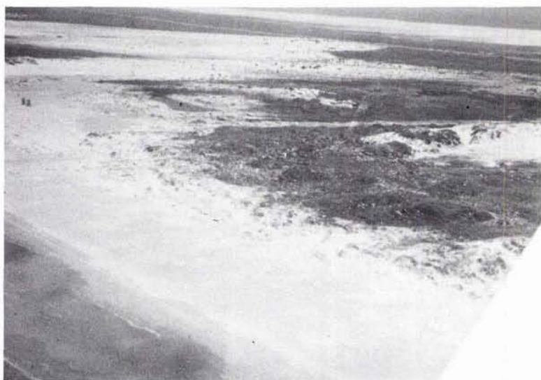
FIG. 9. Areas of different moisture content are delineated on the color-infrared photograph of which this is a black-and-white reproduction. Vegetation is differentiated by intensity of infrared reflectance. In the background, blow-outs taper to the northwest indicating a prevailing southeast wind.
