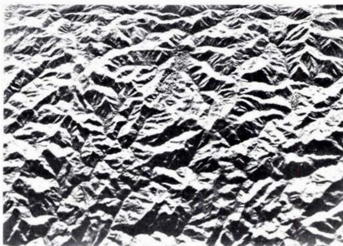
FIG. 10. Radar imagery of Seven Miles Peak ( above ) and Chrome Ridge ( below ) (Onion Mtn., Oregon). Seven Miles Peak area exhibits rounded, difficult-to-define crests, whereas the crests in the Chrome Ridge-Onion Mtn. area are knife-like, easy-to-define crests similar to the type of crests found in the other test areas.
