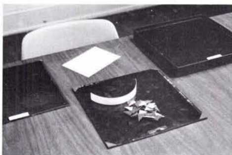
FIG. 2. Adhesive labels can be affixed to the diapositives to facilitate identification. Triangular spacers cut from the adhesive-backed cork strip are stuck to the corners of the plate on the emulsion side to prevent the emulsion from coming in contact with the hot projector top.
