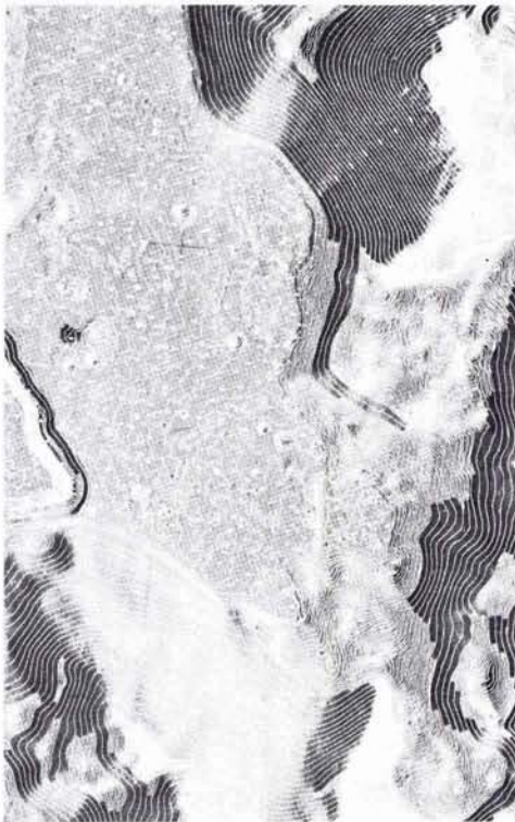
FIG. 10. Composite of panoramic-compiled contours and frame-generated orthophoto.
