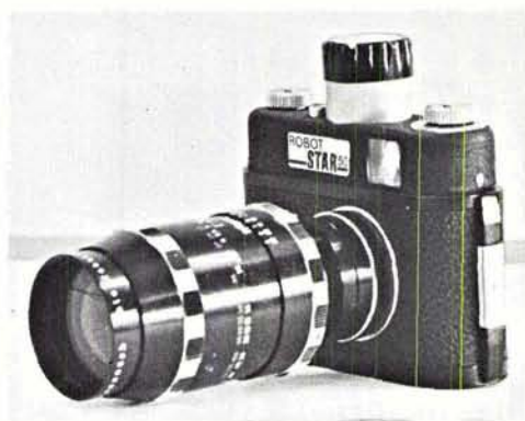
FIG. 1. Robot camera, basic 35-mm film format unit for the multiband-multiemulsion quadricamera, fitted with 150-mm screw mounted telephoto lens for detailed water pollution studies. Robot Star 50 (illustrated), housing on top of camera contains stainless steel spring motor which drives automatic film advance for 50 exposures without rewinding.
