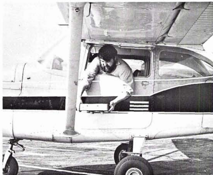
FIG. 4. Operating position of quadricamera for vertical photos from window of light high-wing aircraft. Compact nature of quadricamera allows hand-held use from plane window. The window fastening was modified to allow the window to be opened fully while in flight.
